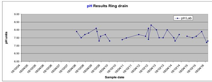
Figure 1: Ring drain pH concentration trend from October 2004 to June 2016
