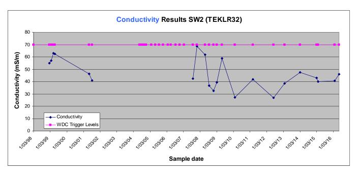
**Figure 2**: Waitomo District Landfill SW2 conductivity results from March 1998 to July 2016 (the pink line indicates the WDC trigger level of 70 mS/m).
