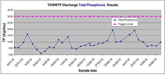
Figure 9- TP Results TKWWTP Discharge January 2016 to August 2016
