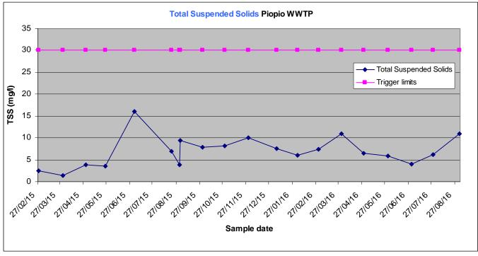
Figure 4 – Total Suspended Solids Results Piopio WWTP
