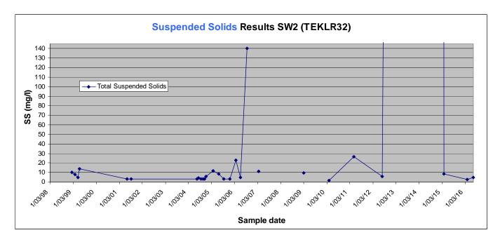
Figure 5: Waitomo District Landfill SW2 Total Suspended Solids Results from March 1998 to July 2016.
