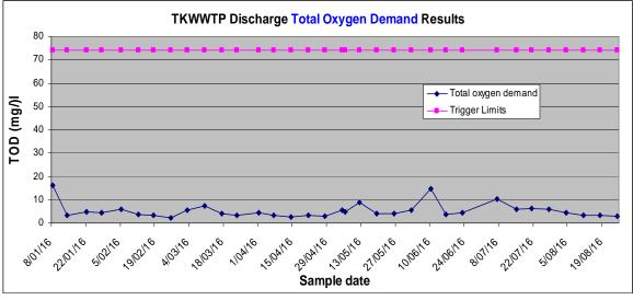
Figure 10- TOD Results TKWWTP Discharge January 2016 to August 2016
