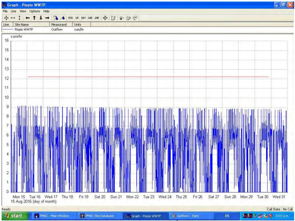
Figure 8 – Discharge flow rate August 2016 (11 m<sup>3</sup>/hr = 3.05 l/s)
