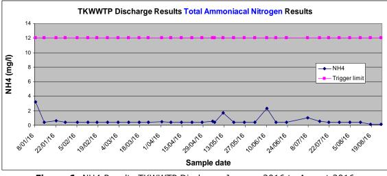
Figure 6- NH4 Results TKWWTP Discharge January 2016 to August 2016
