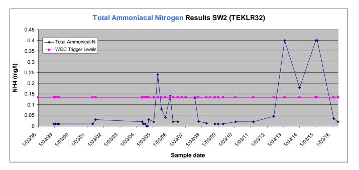
Figure 4: Waitomo District Landfill SW2 total ammoniacal nitrogen results from March 1998 to July 2016 (the pink line indicates the WDC trigger level of 0.13 g/m3).
