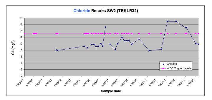
**Figure 3**: Waitomo District Landfill SW2 chloride results from March 1998 to July 2016 (the pink line indicates the WDC trigger level of 13 g/m3).
