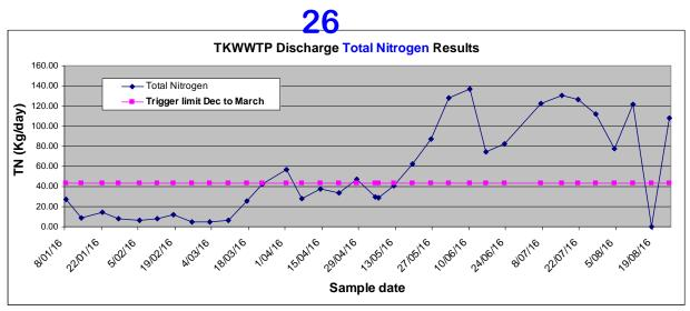
Figure 7- TN Results TKWWTP Discharge January 2016 to August 2016
