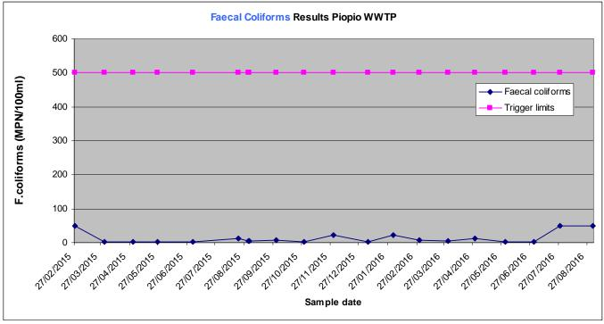
Figure 2 – Piopio WWTP – Faecal Coliform
