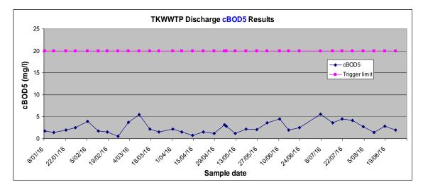
Figure 5 – cBOD5 Results TKWWTP Discharge January 2016 to August 2016
