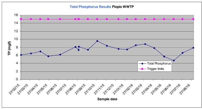
Figure 6- Total Phosphorus Results Piopio WWTP
