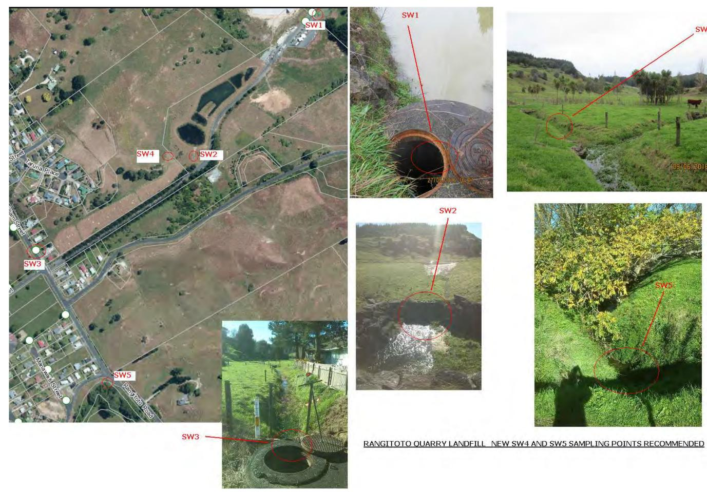
**Figure 3** – WDC Proposed Map for Monitoring Sampling locations with reallocated sampling points SW4 and SW5.
